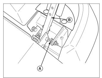
Figure 30. Top Speed Adjustment A. Top Speed Adjustment Bolt B. Control Lever Base
